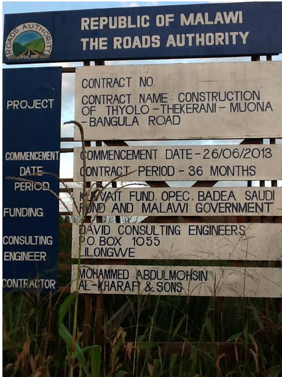
Figure 3-8 Typical example of project sign board providing information to the public
